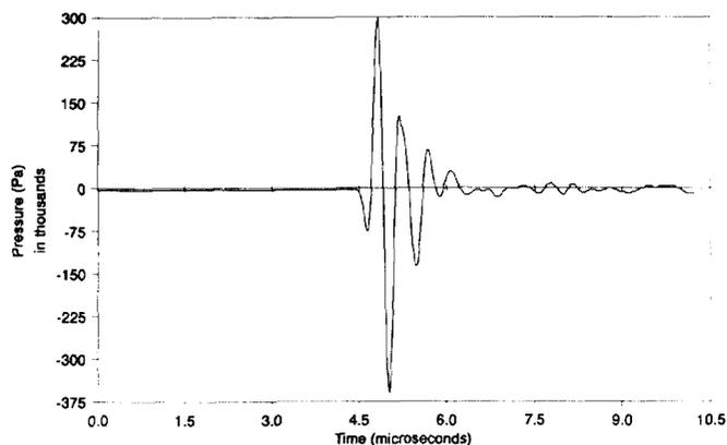
Fig. 5. Calibration pressure waveform, recorded with the same control settings on the B-scanner, with the hydrophone in a water tank.
