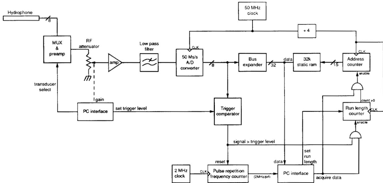
Fig. 1. Block diagram of experiment. Front end of the digital electronics (the trigger comparator and bus expander) is implemented in ECL due to the 50-MHz clock speed. System has no trigger connection to the B-scanner: it is triggered by the ultrasound pulse received by the hydrophone.
