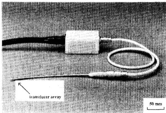
Fig. 2. *In vivo* hydrophone and multiplexer/preamplifier. Side-looking array is positioned at the end of the probe; seven JFET source followers are mounted in the handle.
