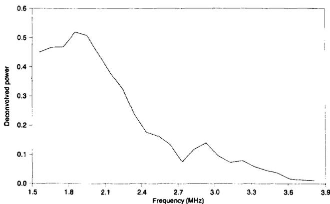
Fig. 7. Ratio of power spectra of *in vivo* and calibration waveforms, showing decreasing sound transmission with increasing frequency.
