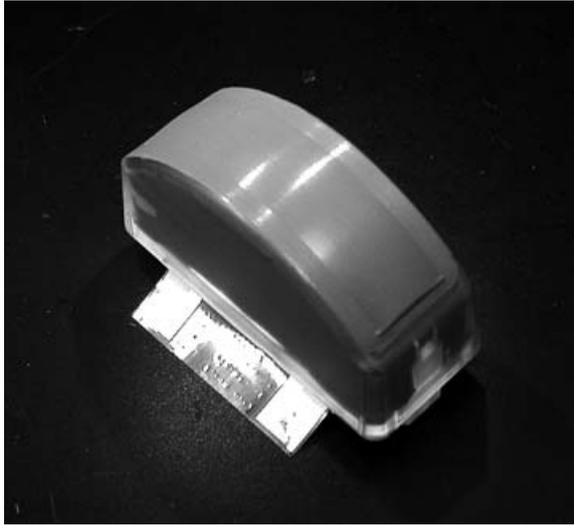
**Figure 1: A 3.5 MHz curved cMUT array with 128 elements and 40 mm radius of curvature.**
